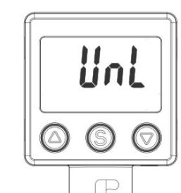
Lock: in the measure mode, press + + button at the same time until "LOC" shown,release the buttons;
