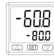
Lock: In the measure mode press at the same time until "LOCK ON" shown, release the buttons
