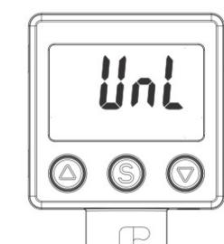
Lock: in the measure mode, press  $\Delta$  +  $\nabla$  +  $\text{S}$  button at the same time until "LOC" shown,release the buttons;
