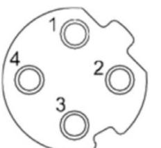
PWR: M12 5PIN plug, A-coded
